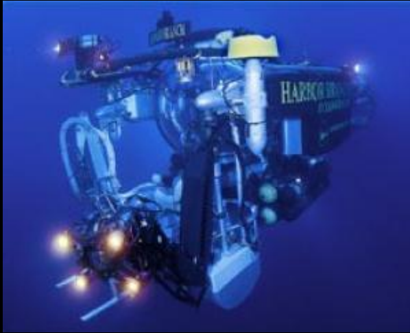
JSL submersible – electric w/ hydraulic capabilities
