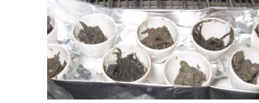
Soil and leaf litter samples are collected along transects and weighed, dried, weighed, combusted. Soil carbon content and moisture are mapped to establish 2-D patterns. A peat corer is used to collect 1-meter cores from which samples are taken for similar analysis down-core.
