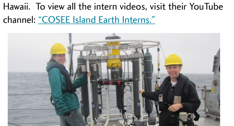
Dr. Judy Lemus and graduate student, Hayley Dosses with a CTD instrument on the R/V Falkor. (Photo credit: Gabi Pilo)
